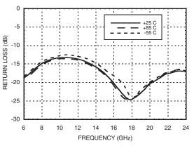
Output Return Loss vs. Temperature
